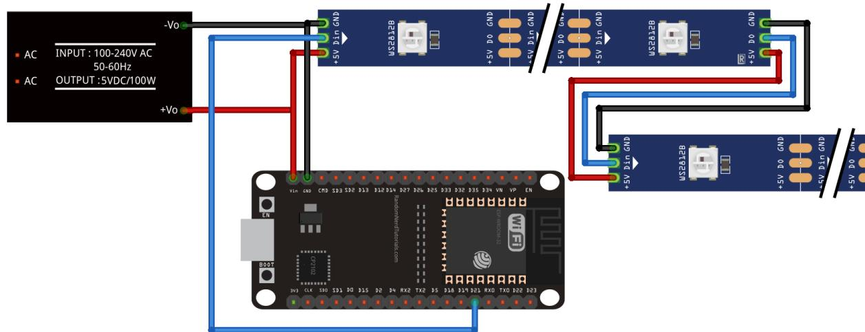
The WS2812B LED Strips should be wired together by connecting the pads like shown on the diagram above. The Connections of the LED strips in the default config is done like this:
